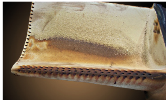
Figure 1: 7FA 1st stage bucket after service
